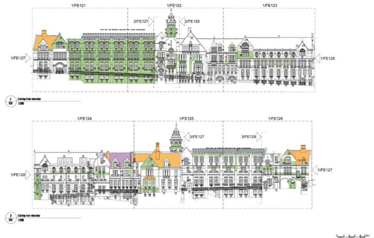
Wall condition: green indicates areas of concrete mortar leading to spalled bricks and deteriorating walls
